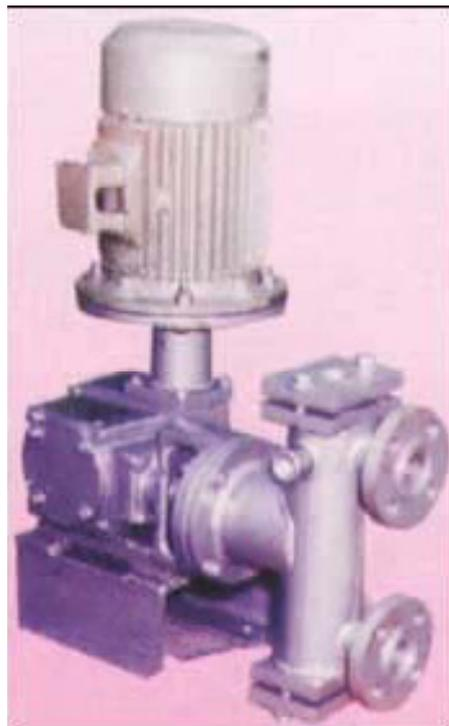
The pump discharge is variable. While pump is running or at rest from zero (0%) to full stork (100%) by means of a precision machined crank equipped with a stork length adjustment mechanism. The stork of the pump controlled either manually (local) or Automatic Electrically (Remote). 4to 20 MA.
