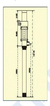
It Eliminate danger of spillage explosion hazard. Construction of Pump is that operating compressed air in contact with pumped liquid. The pump can be directly inserted in to the barrel threading provide on the pump adopter. It sucks the liquid from the bottom and hence less chances of leftover material. It does not have any type of motor and hence virtually zero maintenance.
